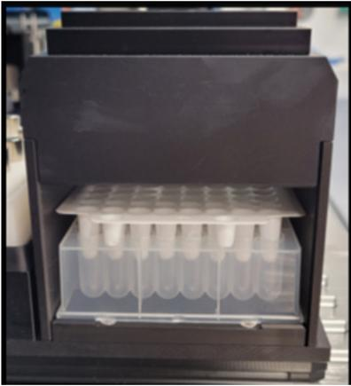
Figure 3: A Protective Plate (Included in the ROBOSCREEN Plate set - INSTANT FX / HMT) allows tips used for buffer transfers to drip-off, which can thereafter be reused to reduce plastic waste.
