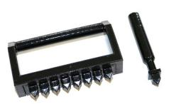
Reagent Plates are prefilled with extraction reagents and are sealed with a foil. Prior to use this foil has to be pierced manually, by using the piercing tools (single piercer or 8fold piercer).
