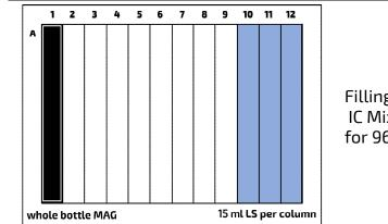
Filling scheme of the R3 - MAG / LS - IC Mix. Depicted is the filling scheme for 96 samples
